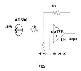
Figure 2. Signal conditioning circuit for AD590
