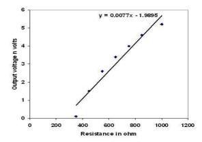
Figure 6. Calibration curve of strain gauge
