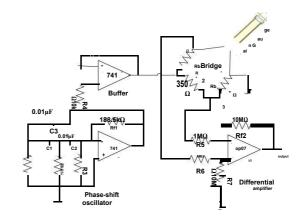
Figure 3. Signal conditioning circuit for strain gauge (part1)
