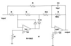
Figure 4. Signal conditioning circuit for strain gauge (part2)
