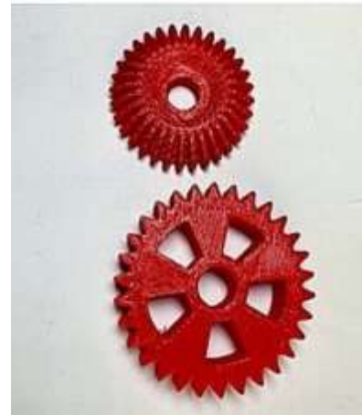
Fig -3 Designed objects printed using 3D printing machine – Bevel and Spur gear
