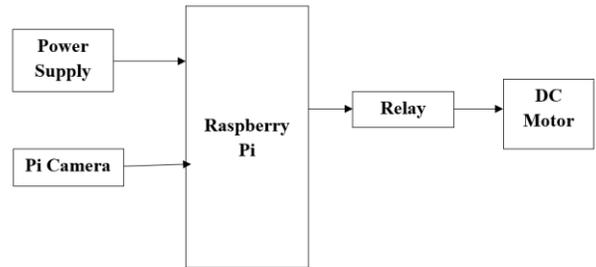
Figure 2: Block diagram for Image processing
