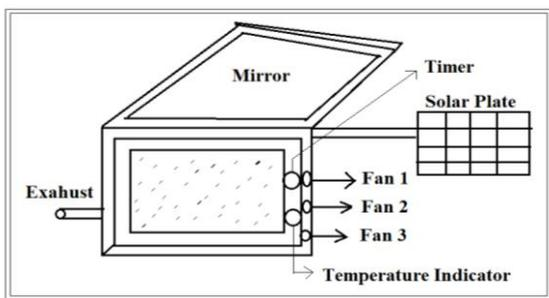
**Fig 3.1: Working principle of in-direct solar drying system**
