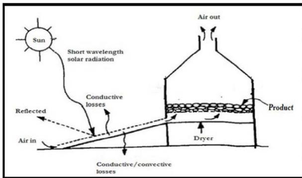
**Fig 1.3 Working of Solar Drying System**
