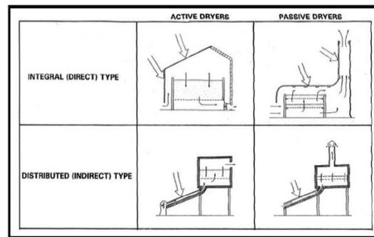
**Fig 1.1 Types of Solar Dryer**
