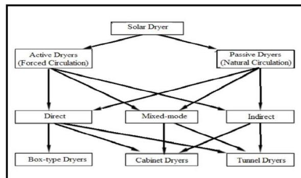
**Fig 1.2 Different groups of solar dryers based on the energy sources used**
