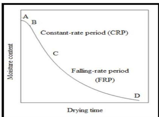
Fig. 3.2. Drying rate curve for a food product
