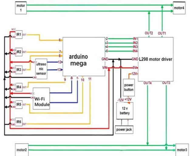
Figure 8: PCB circuit Diagram
