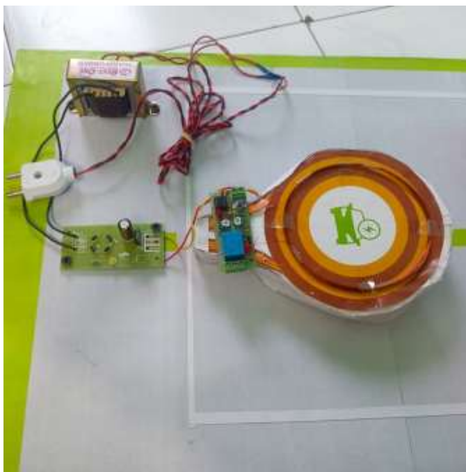
Fig3: Transmitter Side of Project
