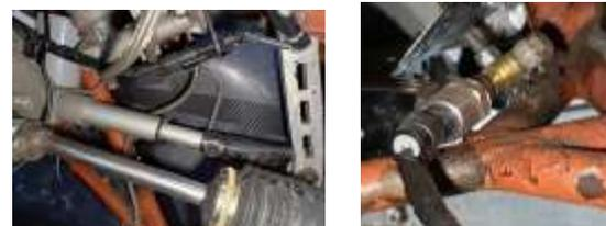
Fig 4: Real time position of our brake actuator and pressure sensor.
