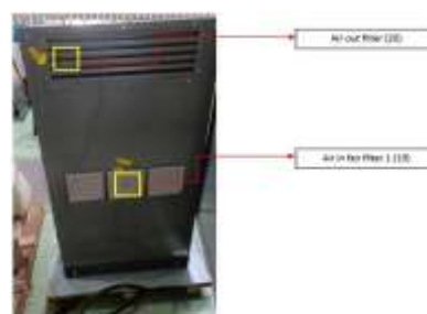
Fig. 8. Rear-panel sensor view — air-in filter (sensor 19) and air-out exhaust filter (sensor 20) thermocouple positions.
