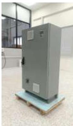
Fig. 5. Fabricated IP54 VFD enclosure prototype -front/side view showing IP54 fan-filter assemblies and door-operated MCCB handle.
