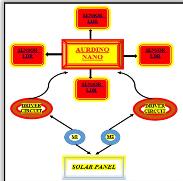
Fig.2: Dual Axis Solar Tracker Block Diagram
