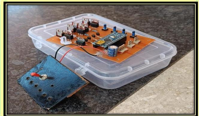
Photograph No.1:- Dual Axis Tracker Circuit
