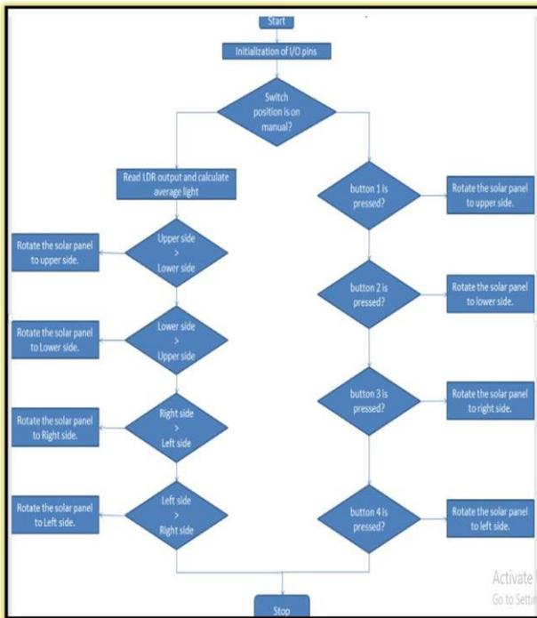
Fig.3: Control Algorithm
