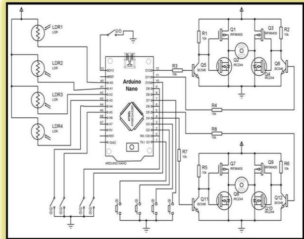
Fig. 1:- Design of Dual Axis Tracker Circuit
