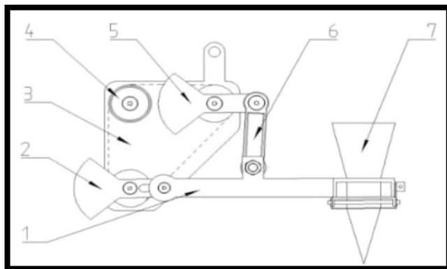
**FIGURE.4.(A) DESIGN OF FIVE-BAR LINKAGE MECHANISM**
