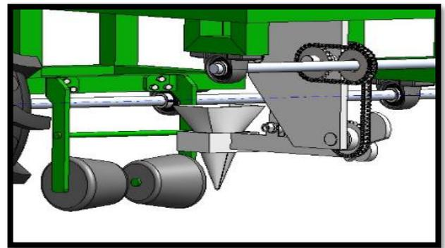
FIGURE.6.(B) 5-BAR LINKAGE MECHANISM
