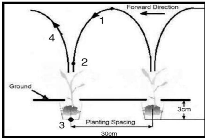
**FIGURE.3.(B) TRAJECTORY OF PLANTING MECHANISM**
