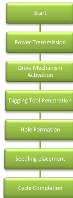
**FIGURE.4.(B) FLOW CHART OF PLANTING PROCESS**
