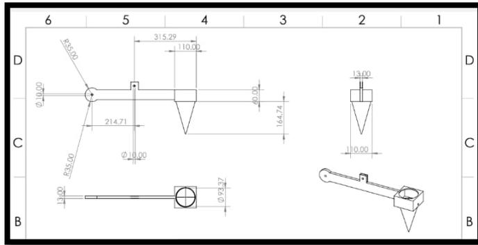
FIGURE.5 DRAFT OF HOPPER UNIT
