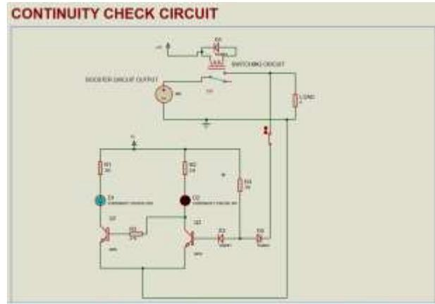
Fig. 8. Continuity Check Circuit
