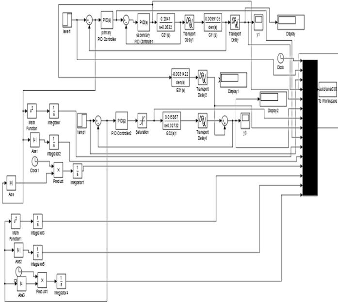
Fig 3 Simulink of PID for operating point 1
