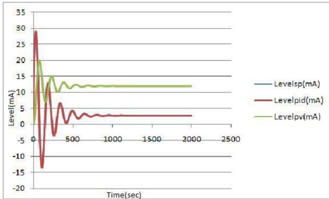
Fig. 7 Response of PID for level
