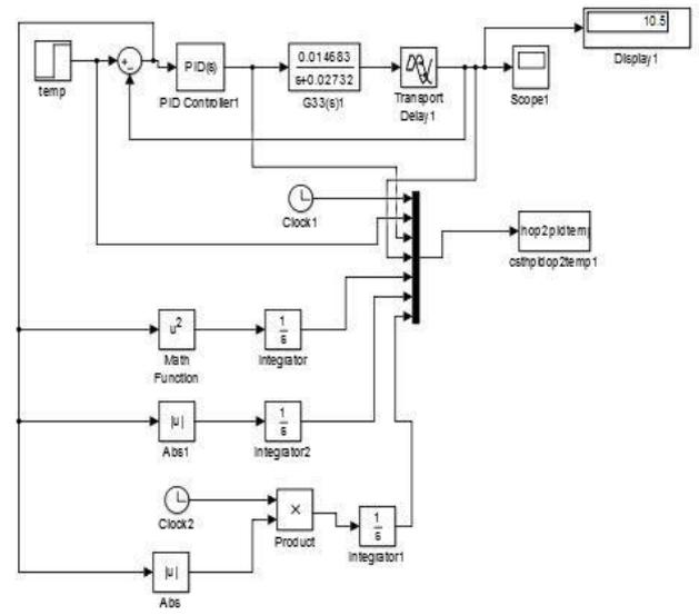
Fig 8 Simulink of PID for Temperature
