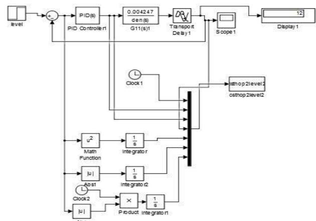
Fig 6 Simulink of PID for level
