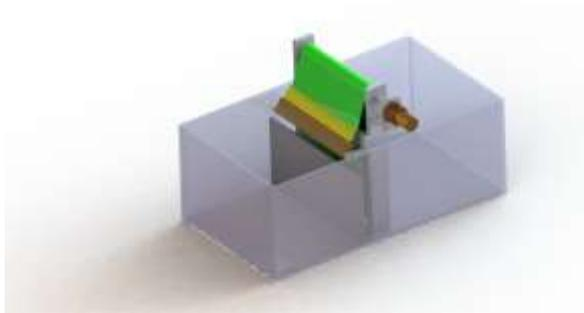
Figure 9: Assembly of Oil Skimmer
