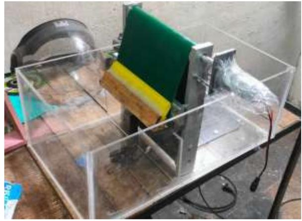
Figure 10: Assembly of Oil Skimmer
