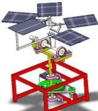
Figure 1. Designed full assembly of the solar smartflower
