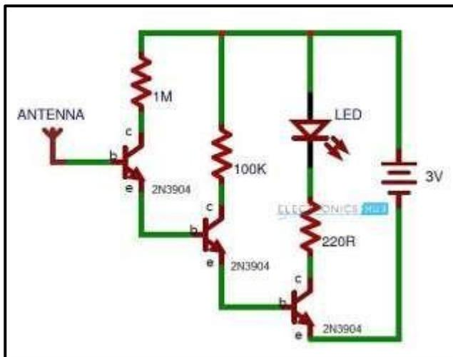
Fig. 5 Circuit diagram for non- Contact voltage detector
