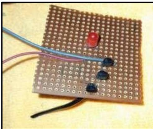
Fig.4: Non- Contact Voltage Detector as Fault Detector
