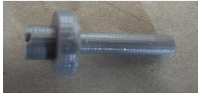
Figure 4.3: 3D printed rectangular nozzle with angle
