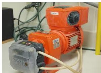
Fig 6.10: Peristillatic pump
