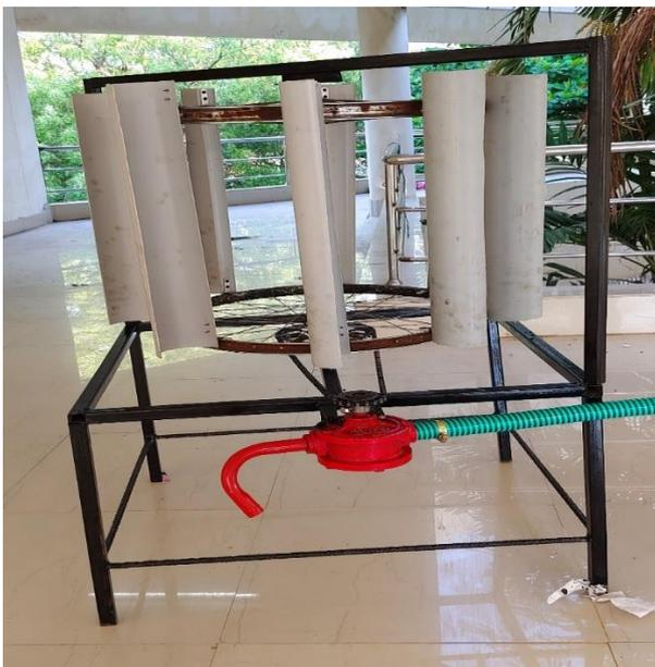
After the installation the experiment examined using the air compressor with wind pressure. The windmill revolutions are taken from non contact type tachometer and the amount of water pumped by the pump is noted at different air pressures. The obtained values are listed out in the table 11.1
