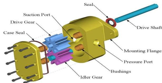
Fig 6.9: Gear pump
