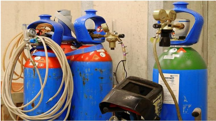
Fig 5.5: Gas welding equipment
