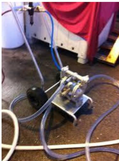
Fig 6.8: Diaphragm pump
