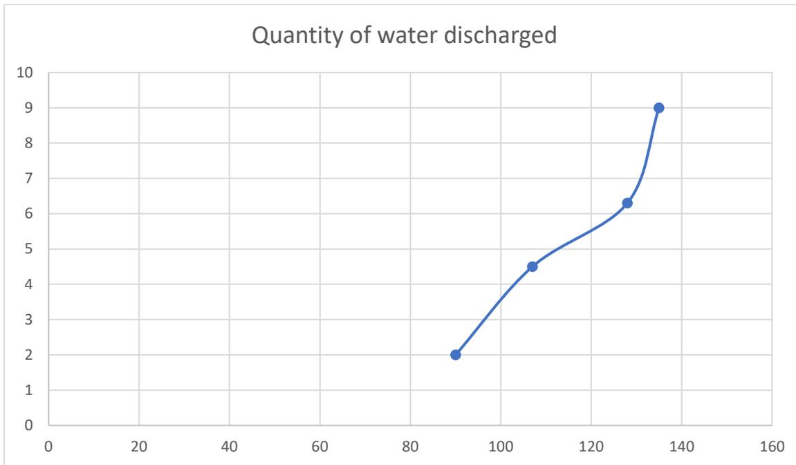
Fig : No of windmill revolutions Vs quantity of water discharged
