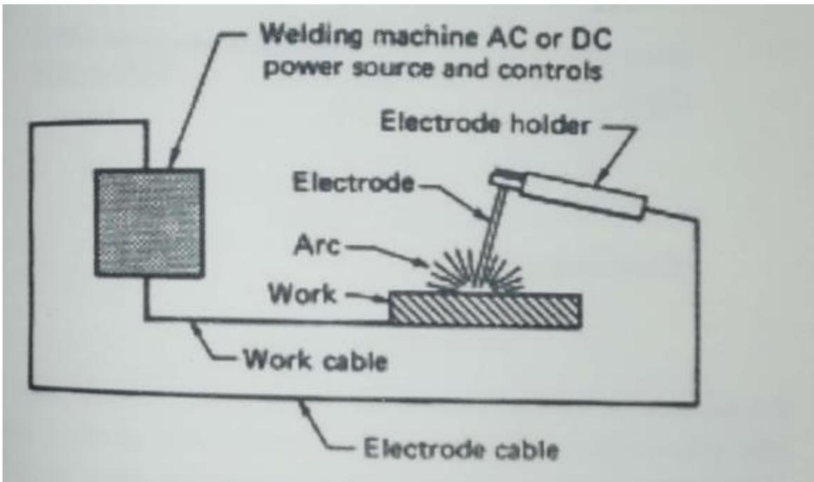
Fig 5.1: Line diagram of Arc welding machine
