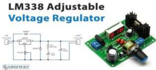
Fig 6. Construction of Regulator
