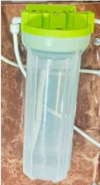
Figure 7. Bubbler unit showing gas inlet and outlet arrangement
