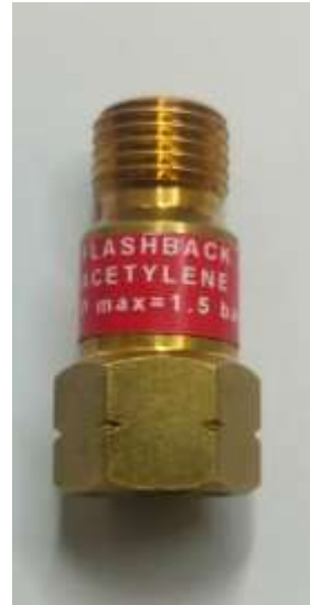
Figure 8. Flashback arrestor used in the hydrogen generator system
