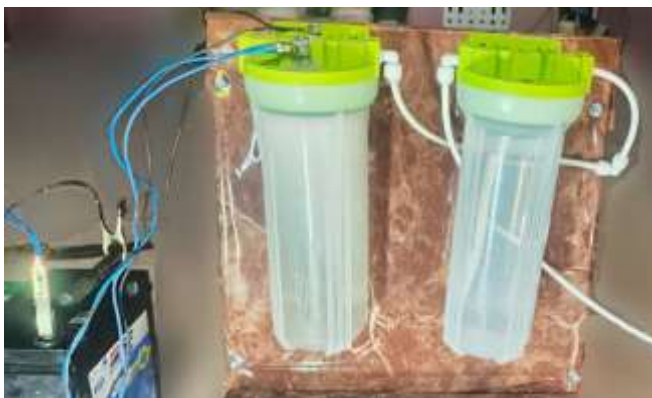
Figure 9. Final integrated hydrogen generator system
