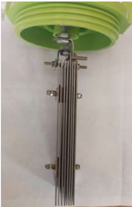
Figure 3. Arrangement of stainless steel electrode plates inside the electrolysis chamber
