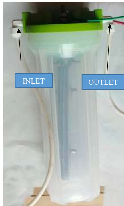
Figure 2. Electrolysis chamber showing inlet and outlet ports
