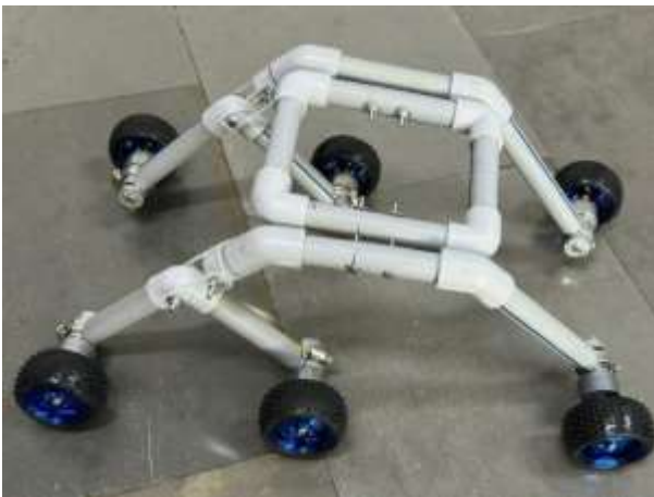
Fig 1: Rocker Bogie made from PVC
