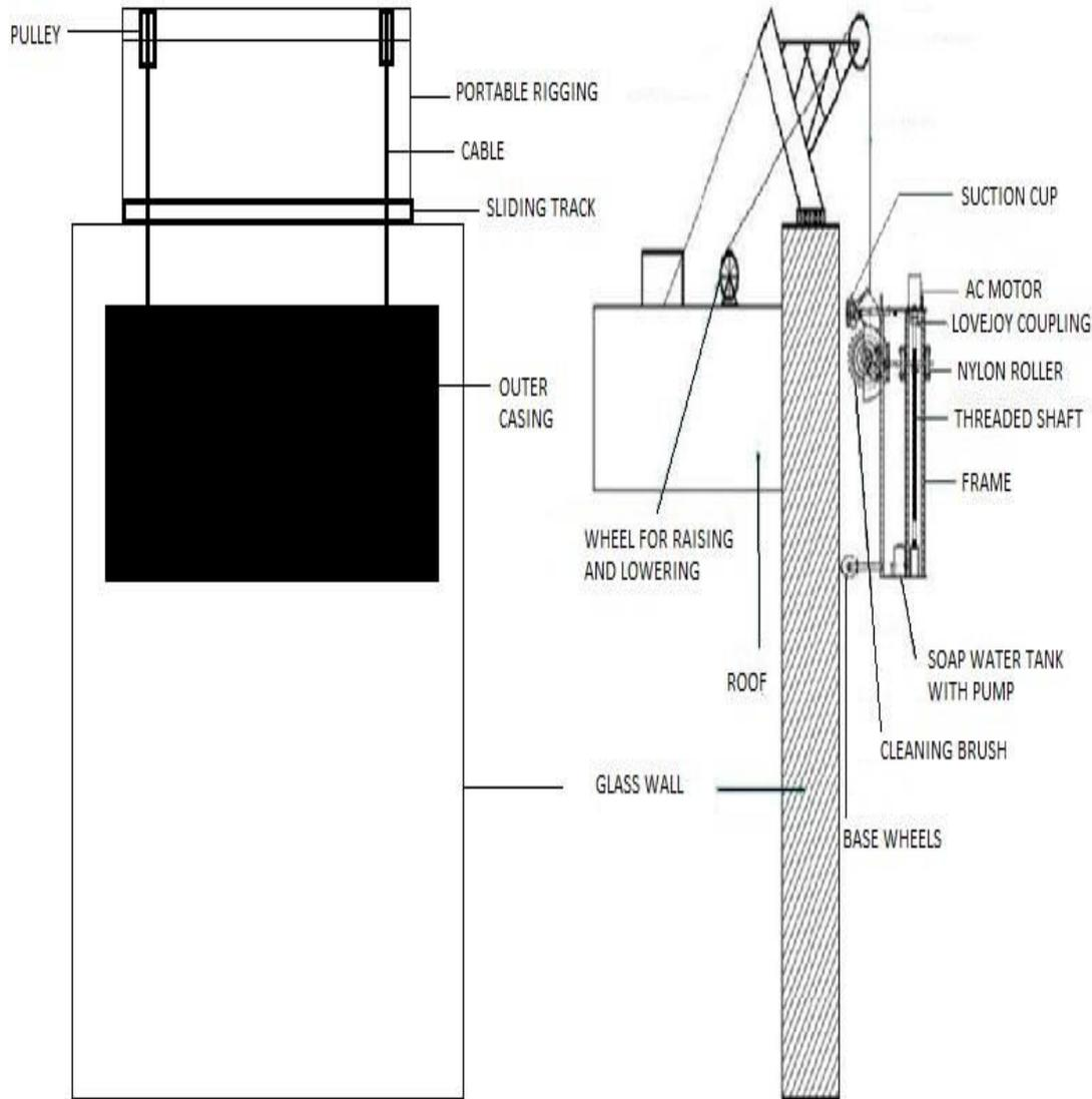
Figure 2: Window Cleaning Machine
