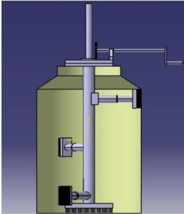
Figure 4. 3D figure of water tank cleaning machine
