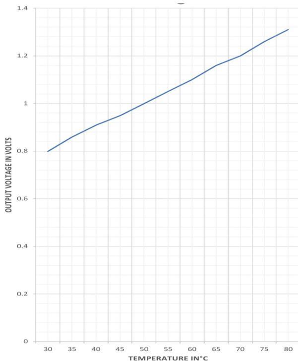
Graph-1 Temperature vs output voltage
