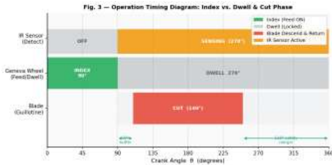
Fig. 3. Operation Timing Diagram — Index Phase vs. Dwell & Cut Phase
