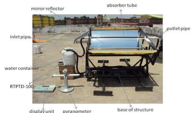
Fig.4 Fabricated parabolic trough solar concentrator for hot water generation.
