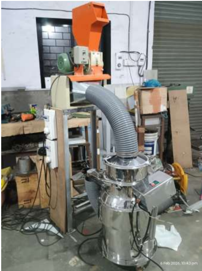
Fig. 2. Plant Assembly showing Flexible Duct Connection and Electrical Control Panel.
