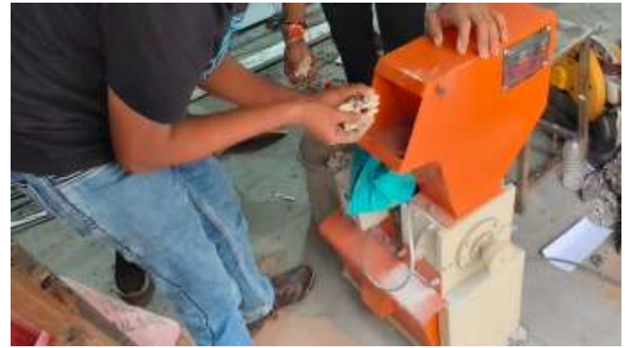
Fig. 1. Primary Crushing Unit with 1 HP Motor and Safety Hopper.
