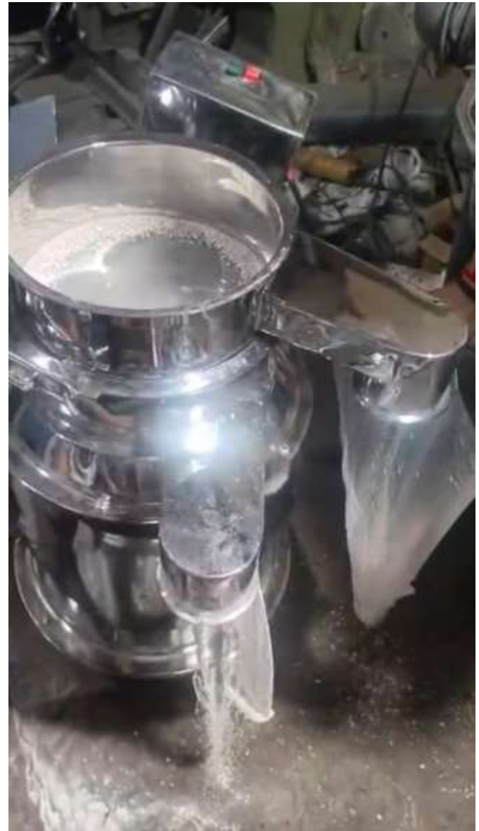
Fig. 3. Stainless Steel Vibro Sifter in operation.
