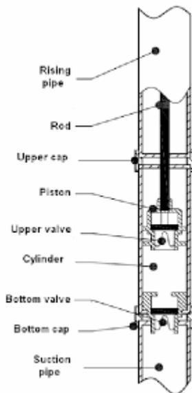
Fig. 3 Cross-sectional model –Single-acting pump
