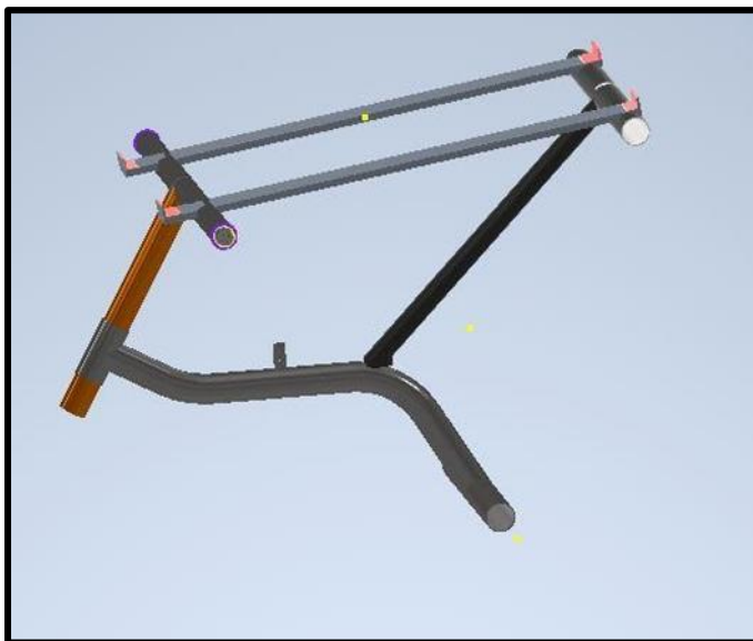
Figure 7 Pesticide Sprayer frame designed in Autodesk Inventor
