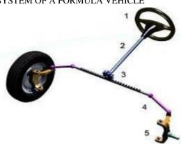
Rack and pinion steering mechanism:
