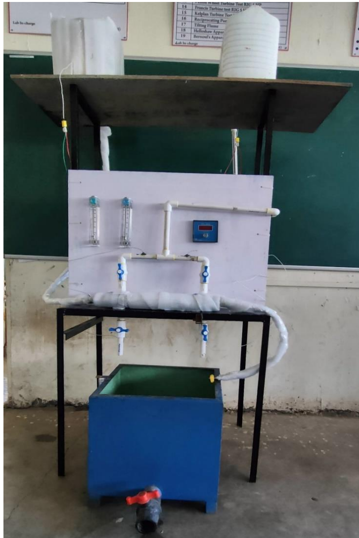
Image. 6.1. TUBE IN TUBE HEAT EXCHANGER
