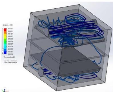
Fig.3.LEDs heat sources simulated at steady state.
