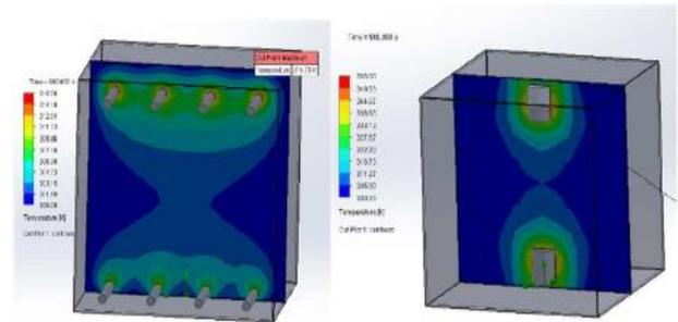
Fig. 4. Thermal simulation results using Solidworks Flow Sim Thermal compare mercury tube (Left) and LED (Right) UV sources to determine fan and air venting requirements.
