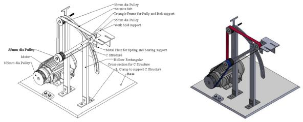
Design modelling of belt grinder using Solid Works:
