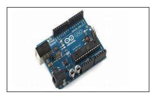
Arduino Uno is open source microcontroller board that helps create interactive projects giving smart solutions by automation. It is based on the processor ATmega328p. It also comes with a variety of input and output pins that can be used to connect different electronic components.
