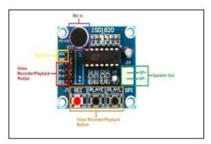
It is a small Voice Recorder and Playback module that can do the multi-segment recording. The user can achieve a high quality of recording (for 8 to 20secs) for each application with the adjustment of the on-board resistor. This Voice Recorder/Playback module is designed with embedded-Flash memory, which can hold data for up to 100 years and erase/record the life cycle up to 100,000.
