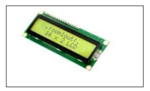
The term LCD stands for Liquid Crystal Display. It is one kind of electronic display module used in an extensive range of applications like various circuits & devices like mobile phones, calculators, computers, TV sets, etc. These displays are mainly preferred for multi-segment light-emitting diodes and seven segments. The main benefits of using this module are inexpensive; simply programmable.
