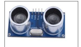
Ultrasonic Sensors are electronic devices that calculate the target's distance by emission of ultrasonic sound waves and convert those waves into electrical signals. The speed of emitted ultrasonic waves traveling speed is faster than the audible sound
