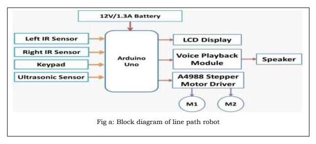
The robot's functionality is divided into the following blocks:
