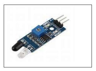
IR sensor is an electronic device, that emits the light to sense some object of the surroundings. An IR Sensor can measure the heat of an object as well as detects the motion. Usually, in the infrared spectrum, all the objects radiate some form of thermal radiation. These types of radiations are invisible to our eyes, but infrared sensor can detect these radiations.
