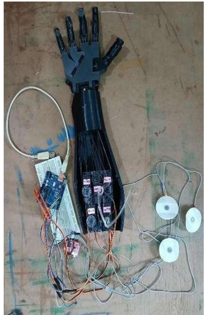
Fig -3: Working Model with components including tendons
