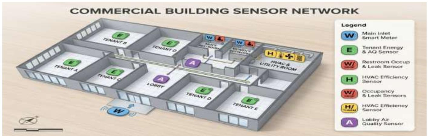
Figure 2: Sensor Placement Schematic
