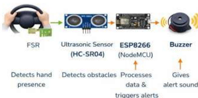
Fig. 3. Modules functionality in the system
