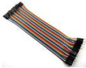
Figure 3.1(e): Jumper Wires
