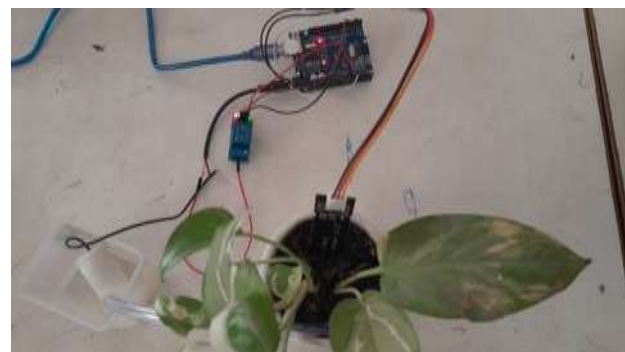
Figure 3.4(a): Implemented Circuit of the Smart Irrigation System
