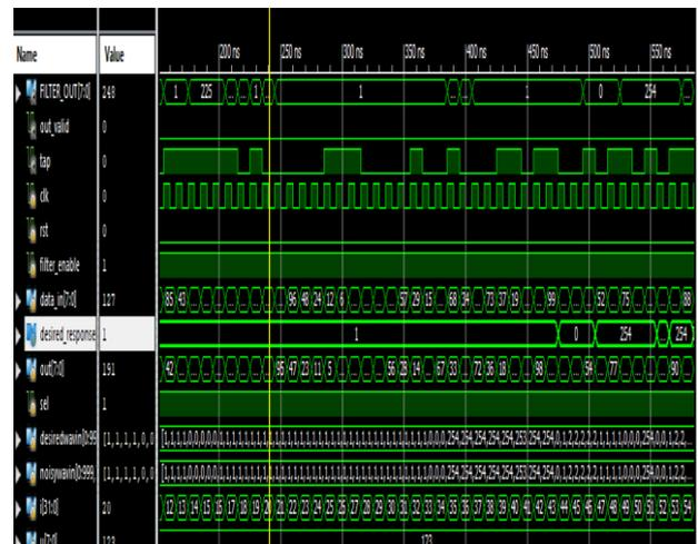
FIG 3: . Simulated results of DA-LUT RFIR on Xilinx.
