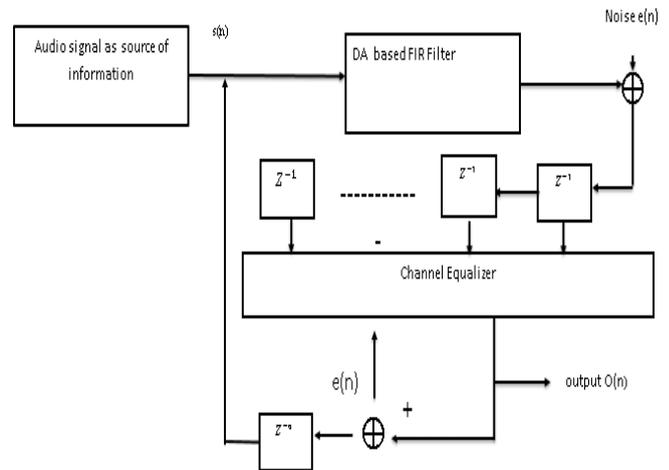
Fig.2.Block diagram of Channel Equalizer of SDR application applied to DA-LUT based RFIR
