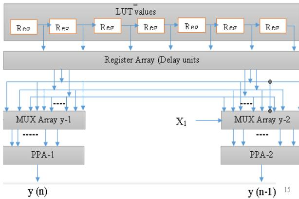
Fig 1.Optimized LUT in DA RFIR filter design
