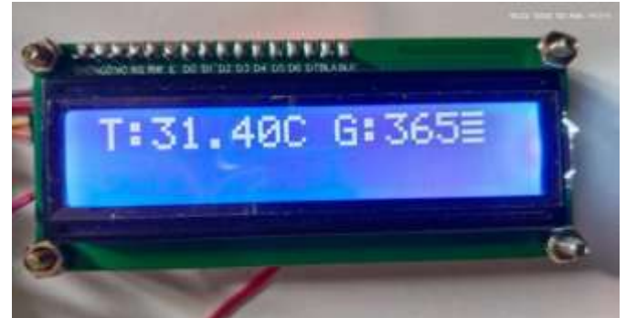
Fig 5.6: LCD Display Showing Temperature Detection
