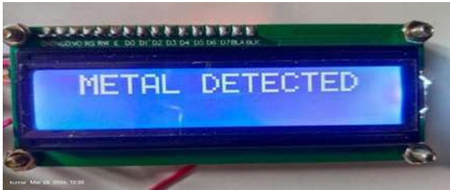
Fig 5.3: LCD Display showing Metal Detection Output
