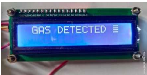
Fig 5.4: LCD Display Showing Gas Detection Output
