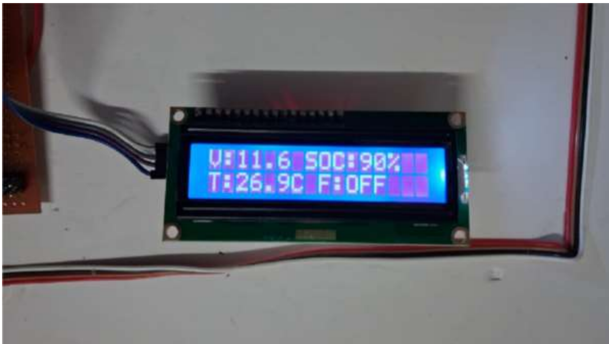
Fig.5 Local monitoring of battery parameters using the 16x2 I2C LCD.
