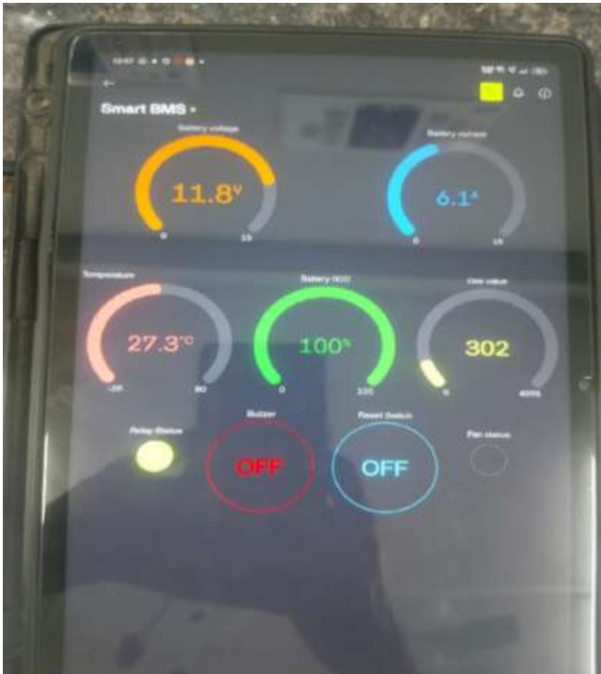
Fig.4 IoT-based remote monitoring and control interface developed using Blynk.
