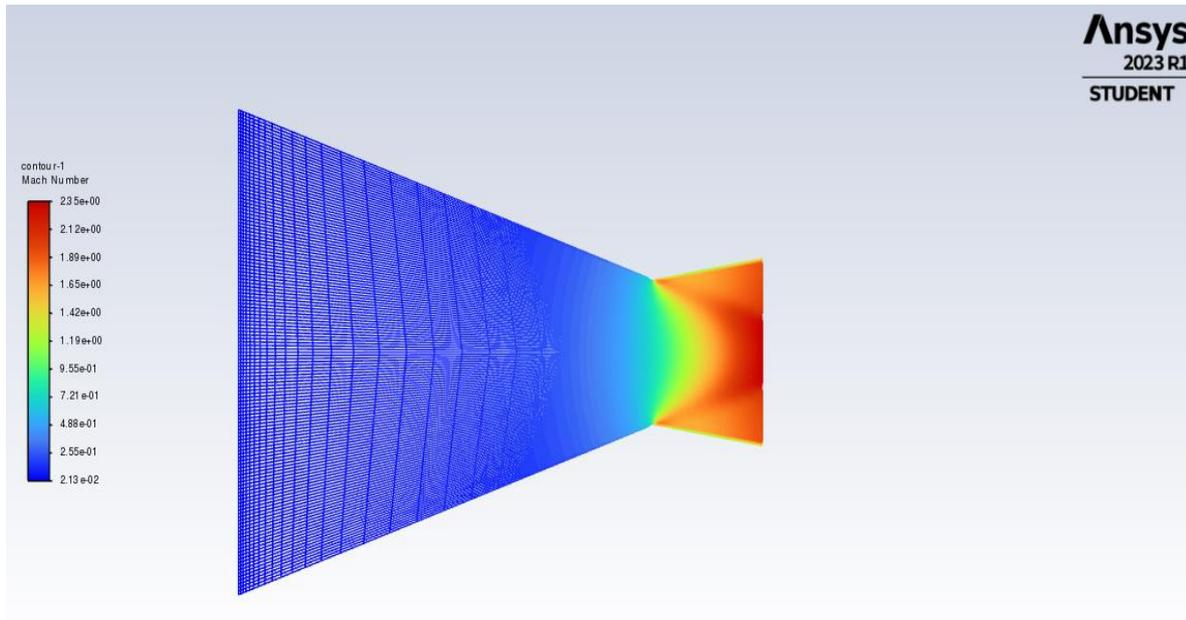
The above figure shows the Mach contour formed for 10° Divergent angle.
