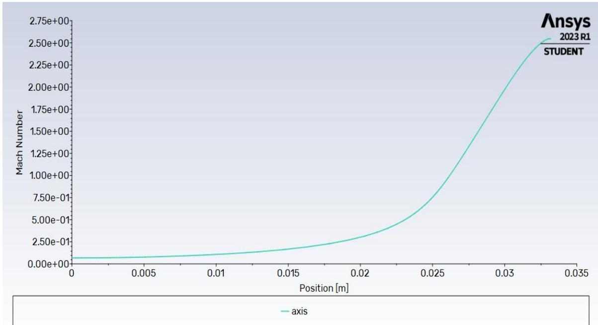
This is the Mach VS Position for shock graph for 8° Divergent angle. It clearly shows that a shockwave is generated just after the exit from the nozzle. This is the optimal condition considering which the nozzle will be designed and manufactured as it shows shockwaves just after the exit condition, the Mach number increases and Static Pressure decreases.
