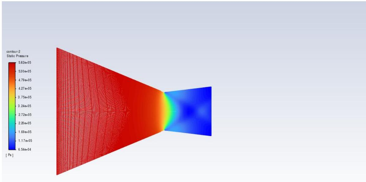
The above figure shows Static Pressure contour for 6° Divergent angle.
