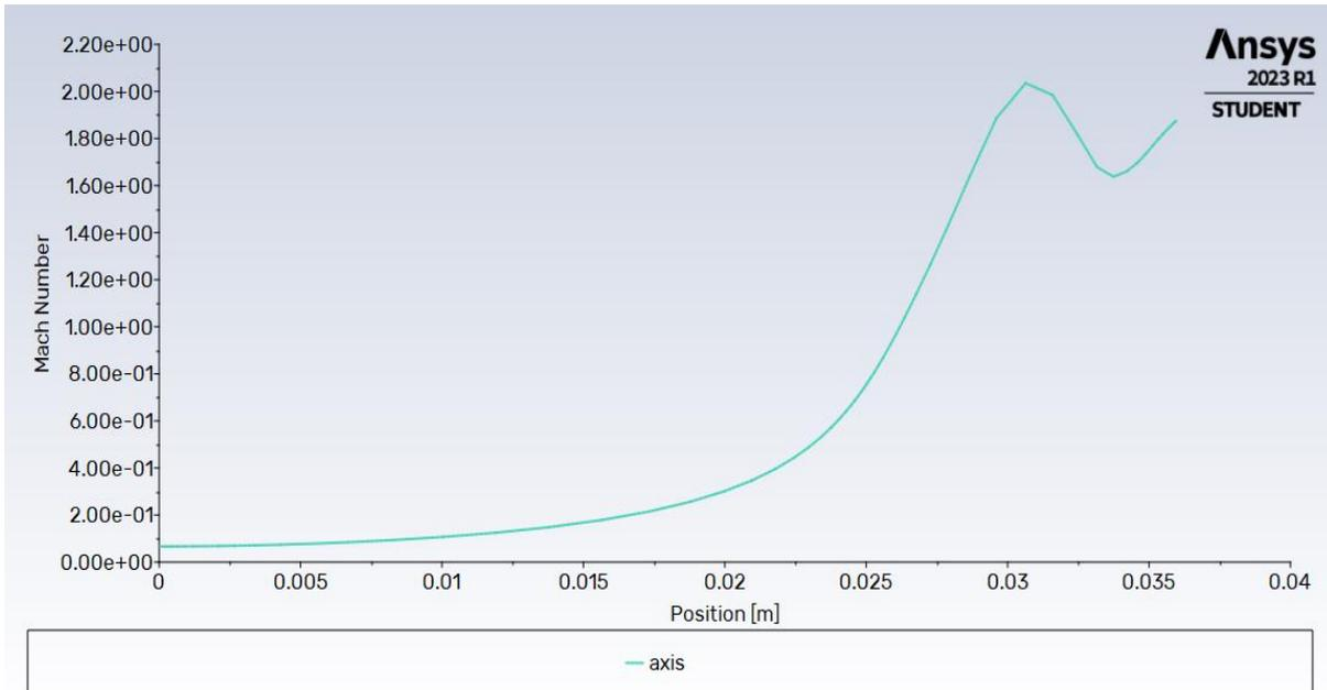
This is the Mach VS Position for shock graph for 6° Divergent angle. It clearly shows that a shockwave is generated at the ending of the Divergent side. The position of the shock is to be seen at 0.0329.
