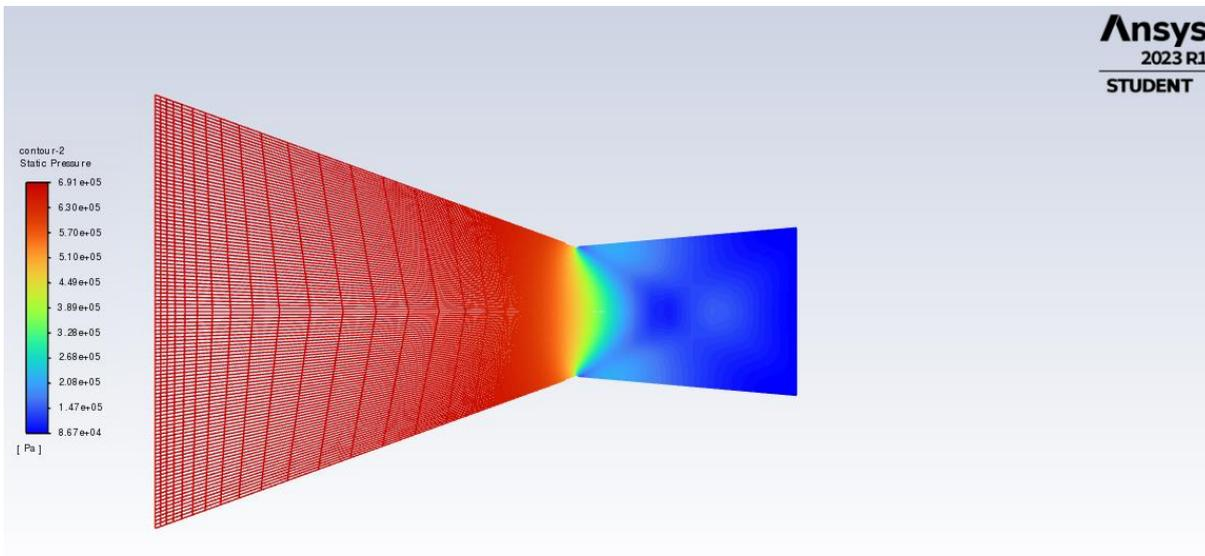
The above figure shows Static Pressure contour for 5° Divergent angle.
