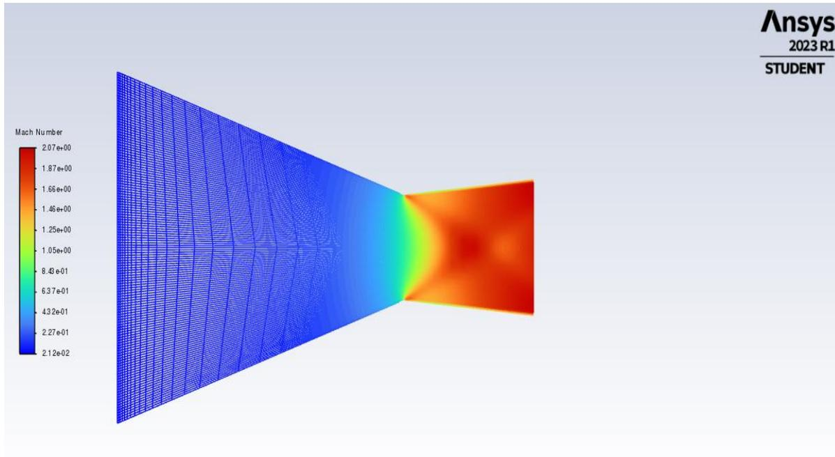
The above figure shows the Mach contour formed for 7° Divergent angle.
