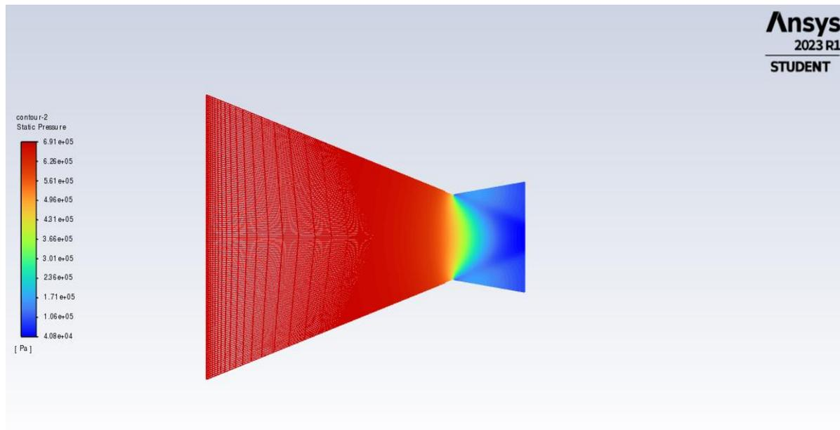
The above figure shows Static Pressure contour for 9° Divergent angle.
