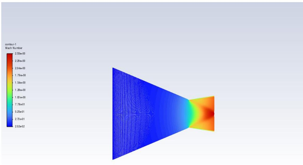
The above figure shows the Mach contour formed for 8° Divergent angle.
