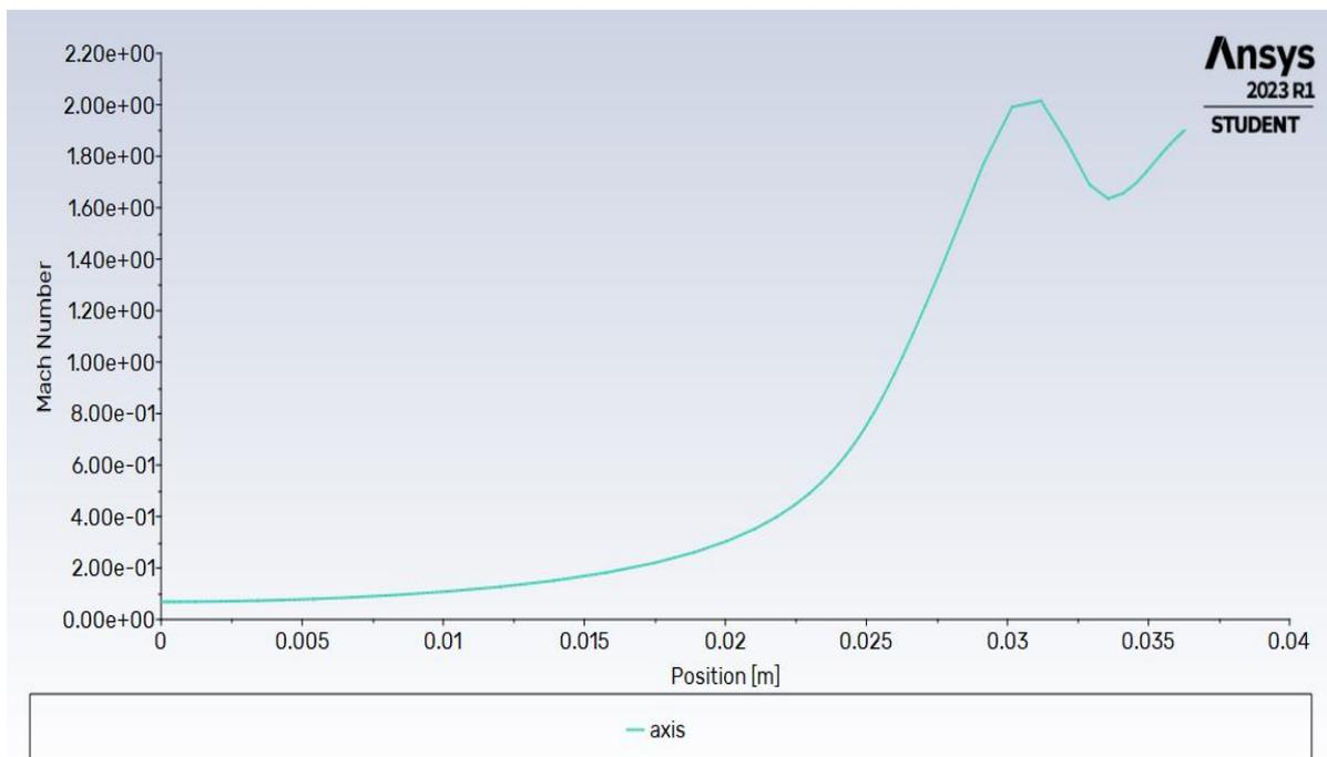
This is the Mach VS Position for shock graph for 7° Divergent angle. It clearly shows that a shockwave is generated at the ending of the Divergent side. The position of the shock is to be seen at 0.0334.
