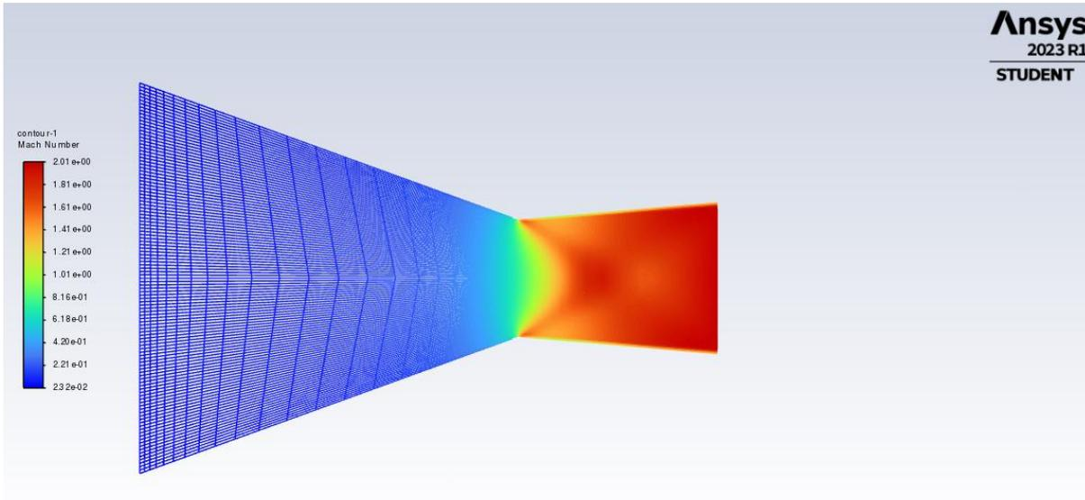
The above figure shows the Mach contour formed for 5° Divergent angle.
