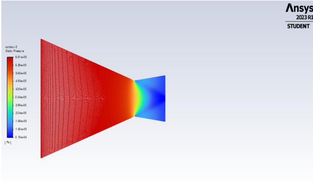
The above figure shows Static Pressure contour for 8° Divergent angle.
