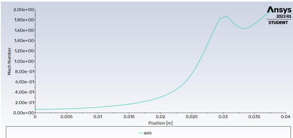
This is the Mach VS Position for shock graph for 5° Divergent angle. It clearly shows that a shockwave is generated at the ending of the Divergent side. The position of the shock is to be seen at 0.0328.
