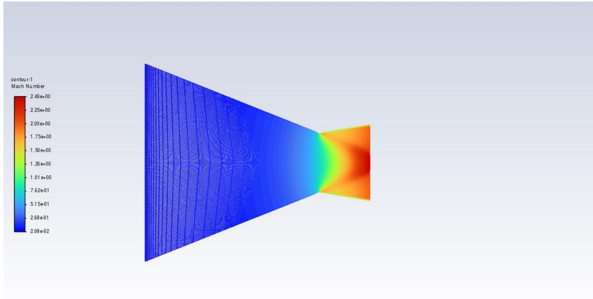
The above figure shows the Mach contour formed for 9° Divergent angle.
