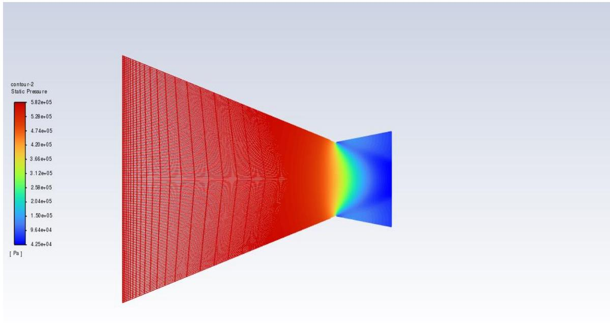
The above figure shows Static Pressure contour for 10° Divergent angle.
