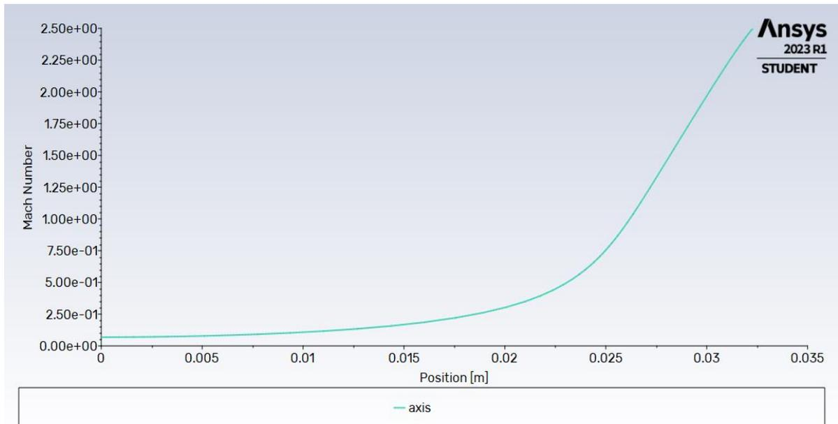
This is the Mach VS Position for shock graph for 9° Divergent angle. It clearly shows that no shockwave is generated.
