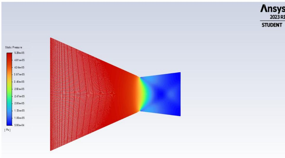
The above figure shows Static Pressure contour for 7° Divergent angle.
