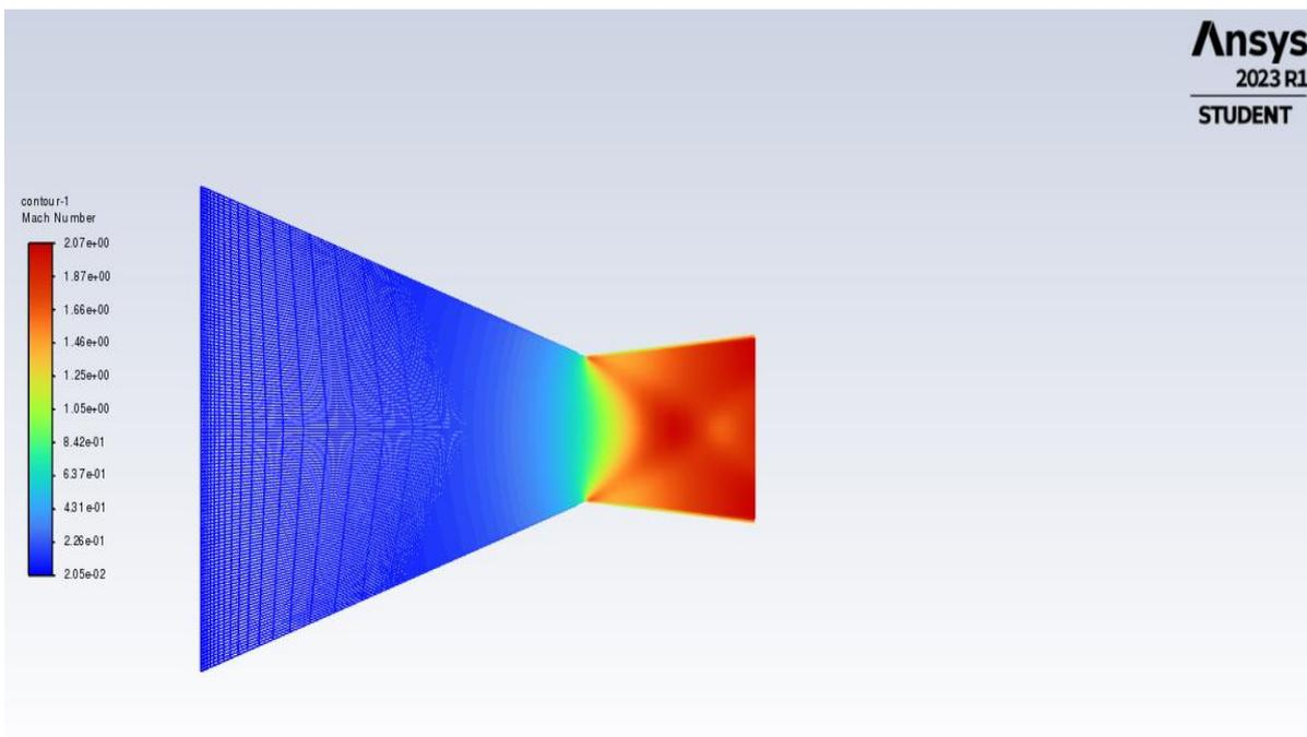
The above figure shows the Mach contour formed for 6° Divergent angle.
