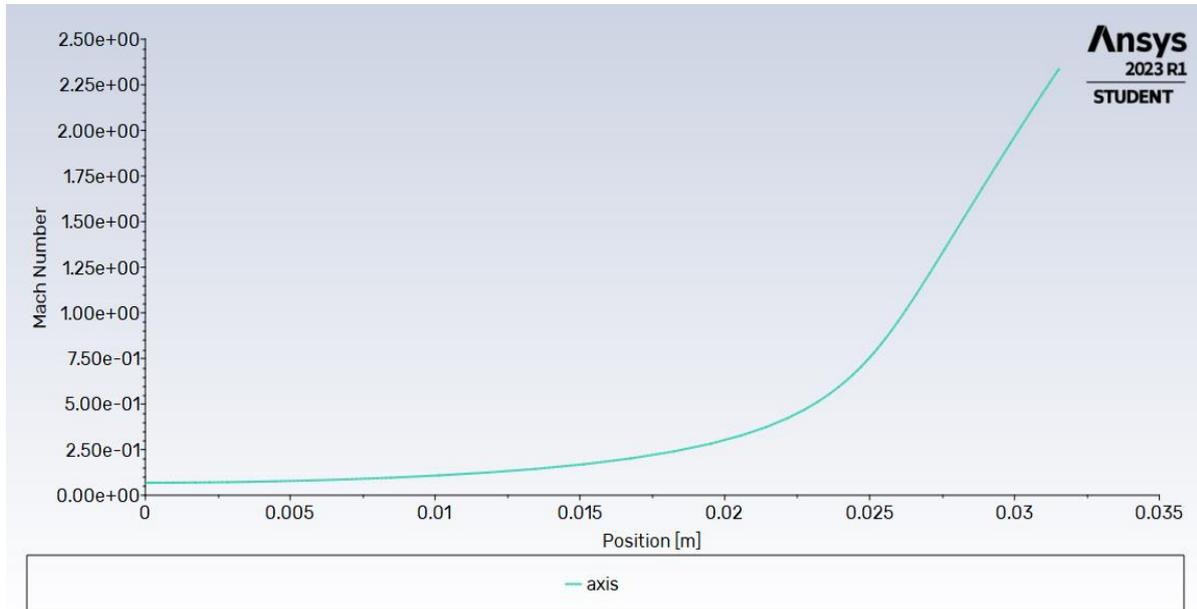
This is the Mach VS Position for shock graph for 10° Divergent angle. It clearly shows that no shockwave is generated.
