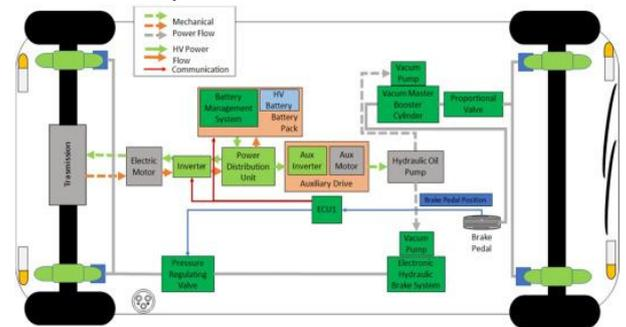
Figure. 2 Structure of Regenerative Braking with characteristics
