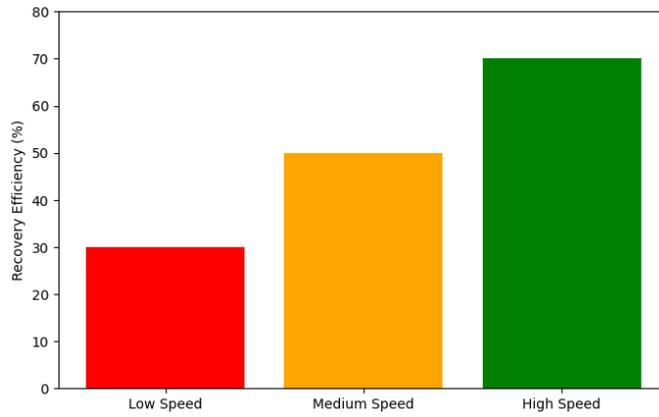
Figure. 3 Energy Recovery Efficiency vs. Vehicle Speed
