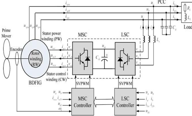
Fig. 1. Configuration of the stand-alone BDFIG system feeding resistive-inductive load.
