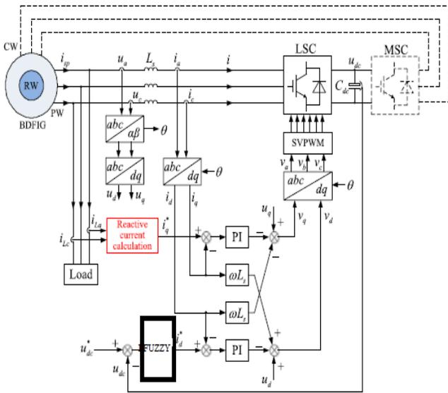
Fig. 2. Control diagram of the LSC with reactive current compensation principle.
