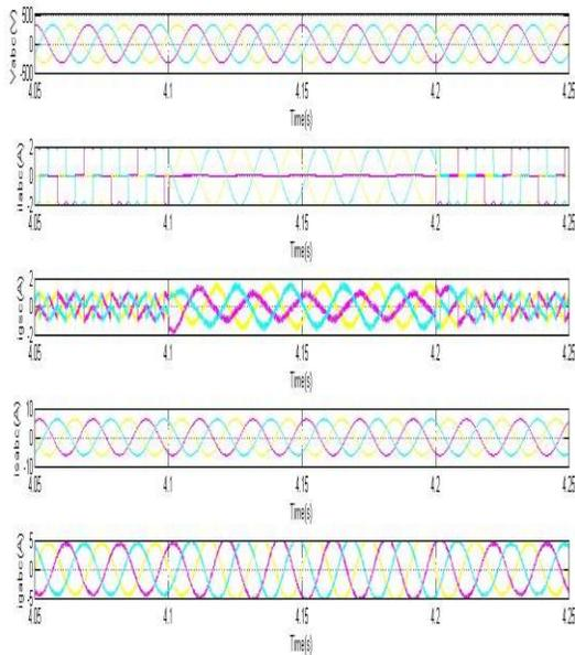
Fig8: Dynamic performance of BDFIG-based WECS for the sudden removal and application of local loads By using fuzzy logic controller
