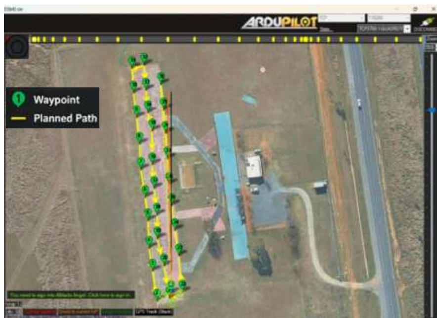
Fig 3: Waypoint mission planning using Mission Planner
