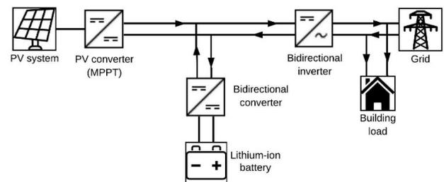
**Figure. 2** Grid-connected PV system with battery energy storage
