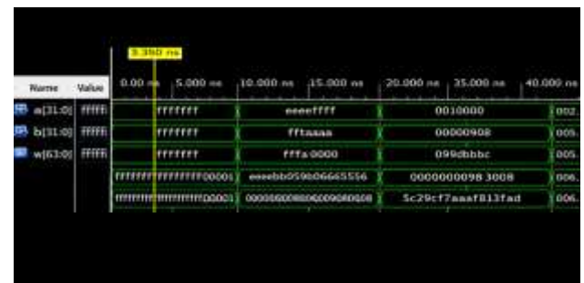
Fig 6: Simulation Results of 32-Bit Vedic Multiplier using Brent-Kung Adder
