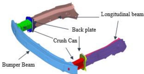
Figure 1. Crash management system (crush can) between main rails and bumper beam [6].
