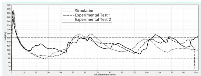
Figure 6. Force-Displacement curve correlation
