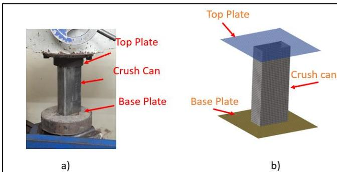
Figure 5. a) Axial load experimental setup, b) Axial load CAE Setup
