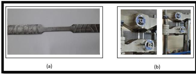
Figure 4. (a) Tensile test specimen, (b) Tensile test setup in UTM
