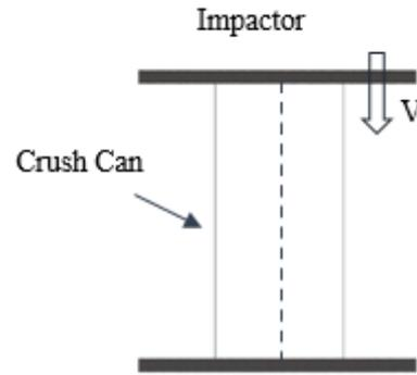
Figure 2. Axial loading of crush can [3].
