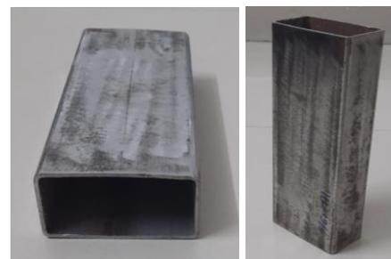
Figure 3. Thin walled tube selected as crush can for experimentation
