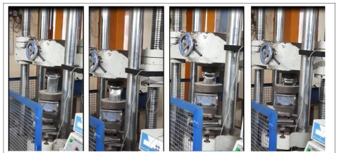
Figure 7. Deformation mode of crush can
