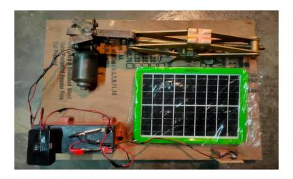
Fig. 1: Diagram of the assembled solar powered Toggle jack
