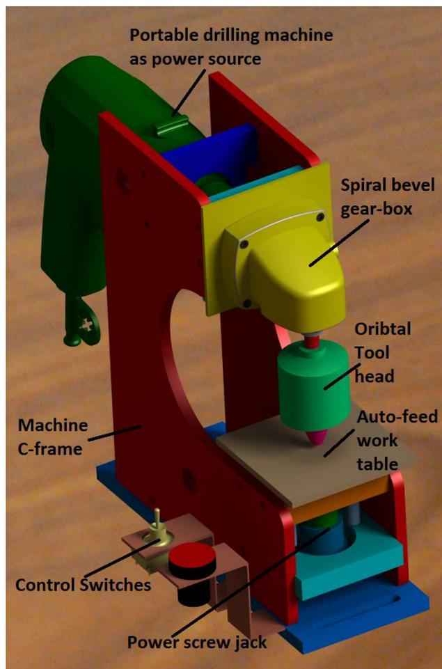
**FEATURES OF PROPOSED ORBITAL RIVETTING MECHANISM**
