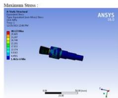
The maximum stress induced is 40.123 MPa is less than permissible stress hence the part is safe
