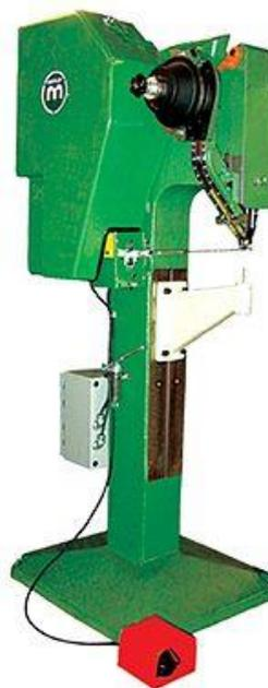
Impact method for solid rivet and semi tubular rivets
