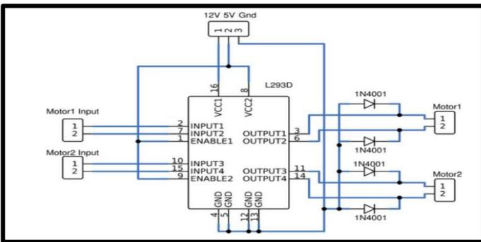
Fig 2: Motor Driver And Motor Connection
